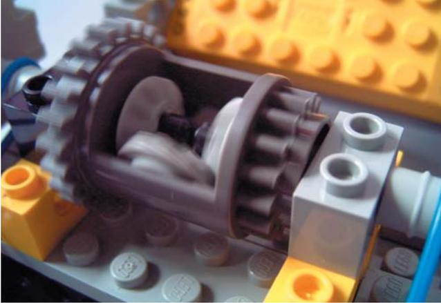
Fig. 1: the differential system to compare two motors
