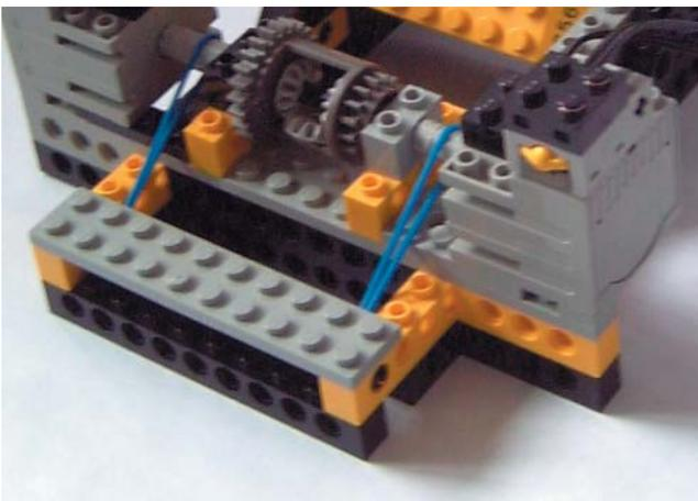
Fig. 6: Supporting parts to keep the motors horizontal
