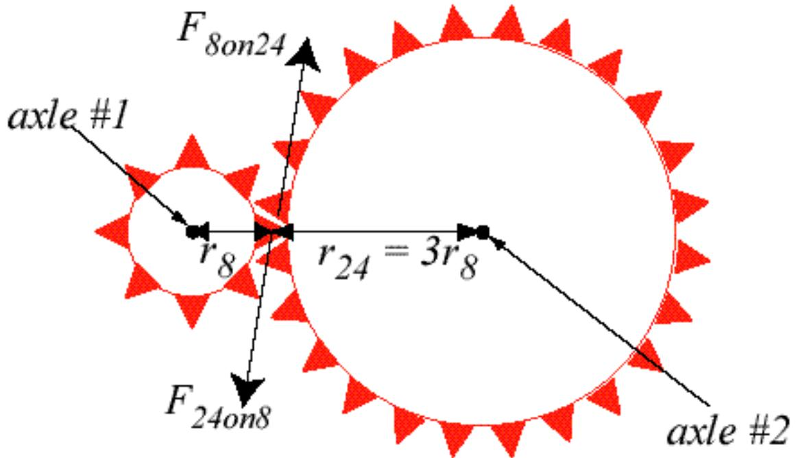
Figure 4 - Since torque =  $r \times F$ , the torque about axle #2 is three times greater than the torque about axle #1; the gear train acts as a "torque amplifier".
