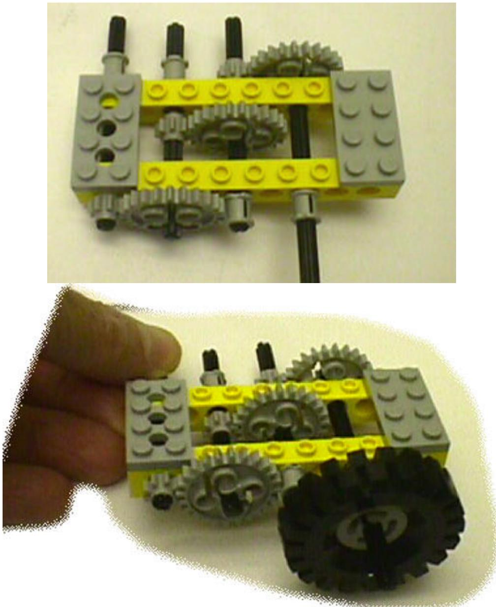
**Figure 6 – A three stage gear train with a gear ratio of 27:1.**
