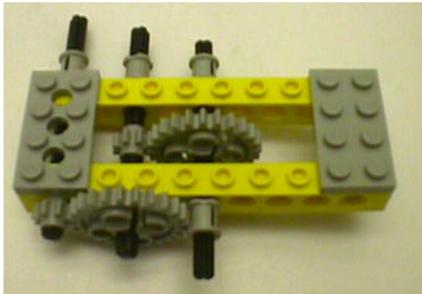
**Figure 5 - By “ganging together” – or multiplying – two 3-to-1 gear reductions, a 9-to-1 output reduction can be achieved. The key is to use intermediary shafts that hold both a large input gear (e.g. a 24-tooth) and a small output gear (e.g. an 8-tooth).**
