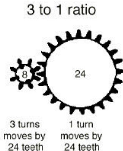
**Figure 3- When the 8-tooth gear rotates 3 times, it advances the meshed gear by a total of 24 teeth. Since the meshed gear has a total, it rotates exactly once. Hence this configuration produces a 3:1 ratio of gear reduction.**
